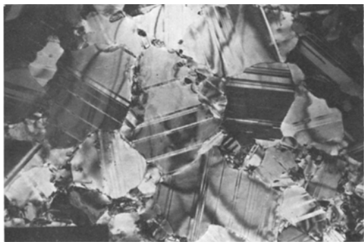
Fig. 2. TEM photograph of nickel coating with texture \langle 211 \rangle (X 13 000).
